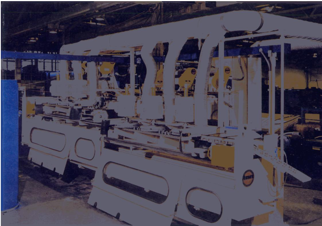
**Figure 8: Automated disc brush deburring system**
