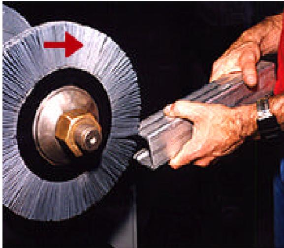
**Figure 1** Off-Hand Deburring of an Aluminum Extrusion
