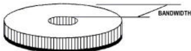
**Figure 6** Band Width of Disc Brushing Tool
